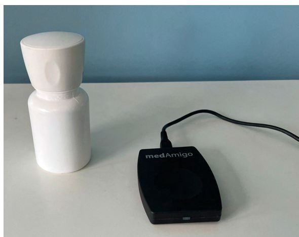
Figure 1. The medication Adherence Monitoring System (MEMS), consisted of an electronic cap, medication container, and a reader, enabling the programming of the device as well as transferring the adherence data
