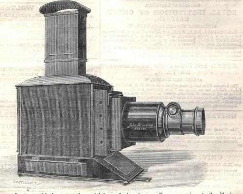
The new Compact Lantern, with the patent three-wick lamp, for burning paraffin or any mineral oil, will give at least 50 per cent. more light than any lamp previously introduced. The lamp burns without a chimney, and the Lantern will give an excellent picture up to 10 ft. diameter.
