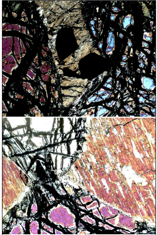
Fig. 4. Typical peridotites from Oulu (up - thin section, down - polarized light).
