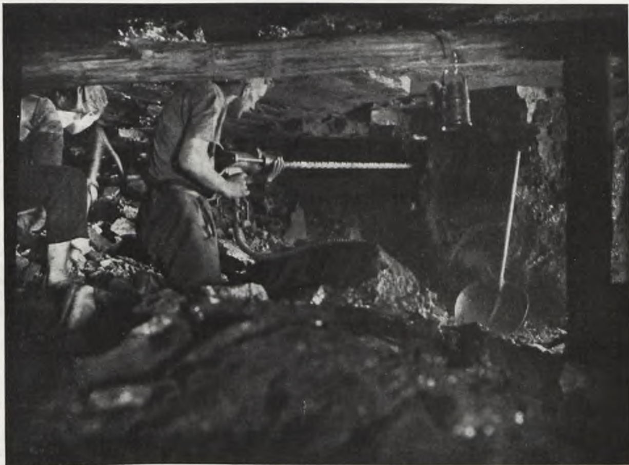
USING A PNEUMATIC DRILL AT THE HOYM MINE, UPPER SILESIA (PHOT. S. PLATER)
