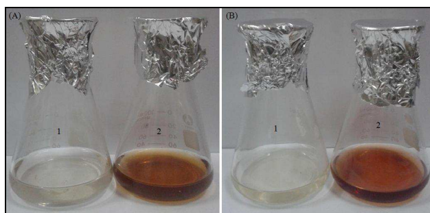
Figure 1. Change of color from pale yellow to brownish, indicating the formation of silver nanoparticles, (A) N. novaehollandae cell filtrate (1) without \text{AgNO}_3 and (2) with \text{AgNO}_3 , (B) T. inhamatum cell filtrate (1) without \text{AgNO}_3 and (2) with \text{AgNO}_3 .
