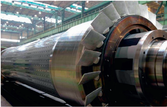
Photo 1. The new turbogenerator rotor fans
