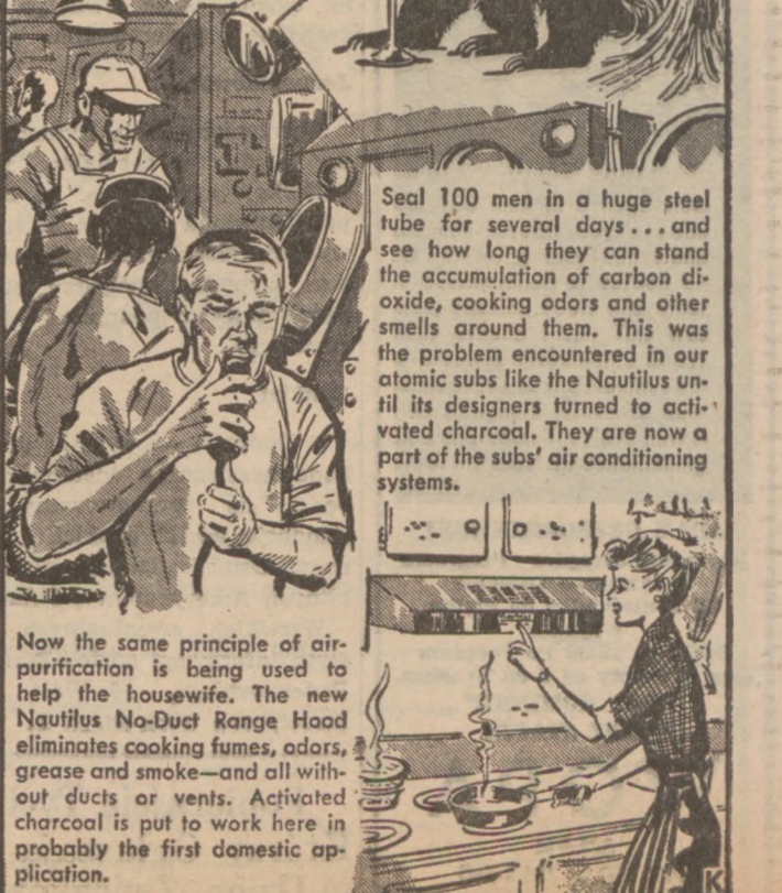
Seal 100 men in a huge steel tube for several days... and see how long they can stand the accumulation of carbon di- oxide, cooking odors and other smells around them. This was the problem encountered in our atomic subs like the Nautilus until its designers turned to ac- tivated charcoal. They are now a part of the subs' air conditioning systems.
