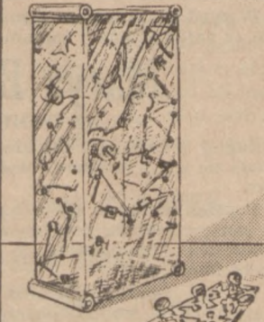
SOLID STATE — many electronic components, excluding vacuum tubes, joined together or cast in a solid block of plastic providing low temperature microcircuits.
