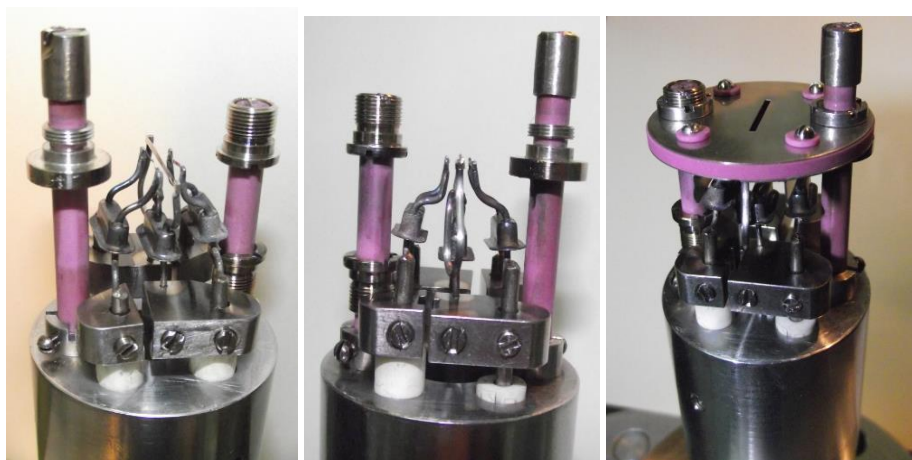
Figure 1. Triple filament ion source of TIMS with wide ionization filament (Pt/Ir) between evaporation filaments (Rh).
