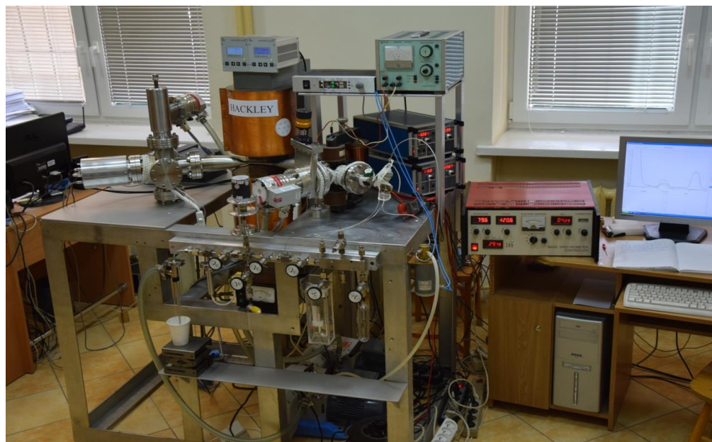
Figure 1. Overall view on the 60° magnetic sector mass spectrometer. The dual inlet system is installed at the front panel. The ion source is on the right side and the collector assembly on the left of the flight tube. The recording of mass spectra and the analysis of isotope ratios are computer controlled.
