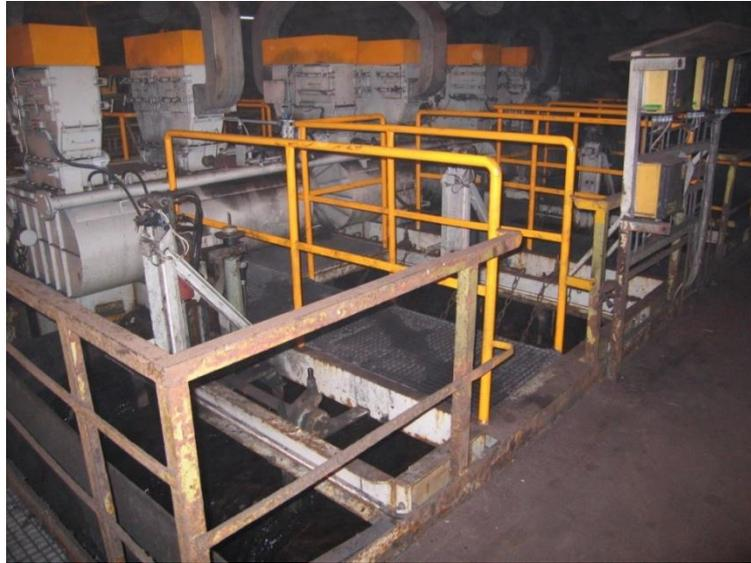
**Fig. 1.** OS26D3E medium-size-grain jig
