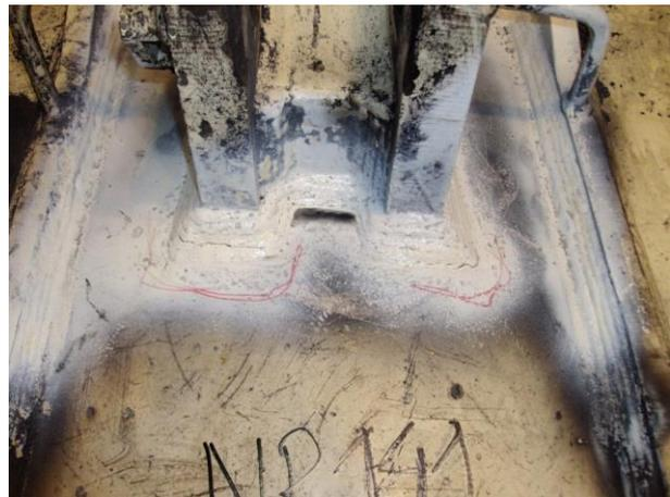
**Fig. 2.** Damaged welds in the gob shield of roof support No. 135[12]
