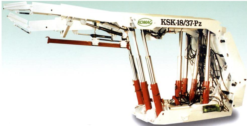
**Fig. 4.** KSK-18/37-Pz mechanized crossing unit [15]
