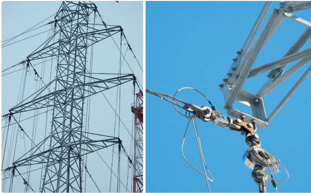
Photo 1. A support prepared for the strength test, set with ropes and signal wires
