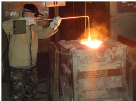
Fig. 4. Experimental-industrial test of installation of advanced derivational thermal express analysis of quality of liquid iron in induction medium-frequency furnace (160 kg)
