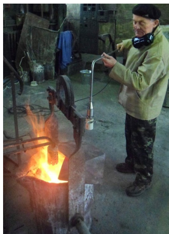
Fig. 5. Pilot-industrial test of installation of advanced derivatized thermal express analysis of quality of liquid iron as applied to transport-melt ladle
