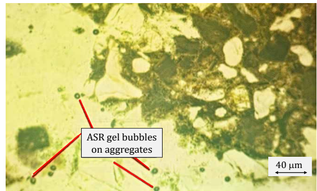
Fig. 6. Petrographic images at 30% CBA replacement
