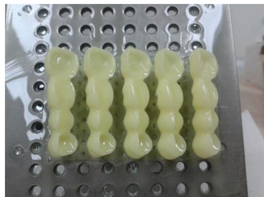
Fig. 1. 3D printed cast patterns of dental bridges [3]
