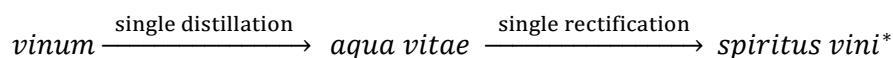
Fig. 1. Processes of distilling and rectifying wine. *Synonyms: spiritus vini = aqua vitae rectificata (PhHis1794:101, PhHis1826:200).
