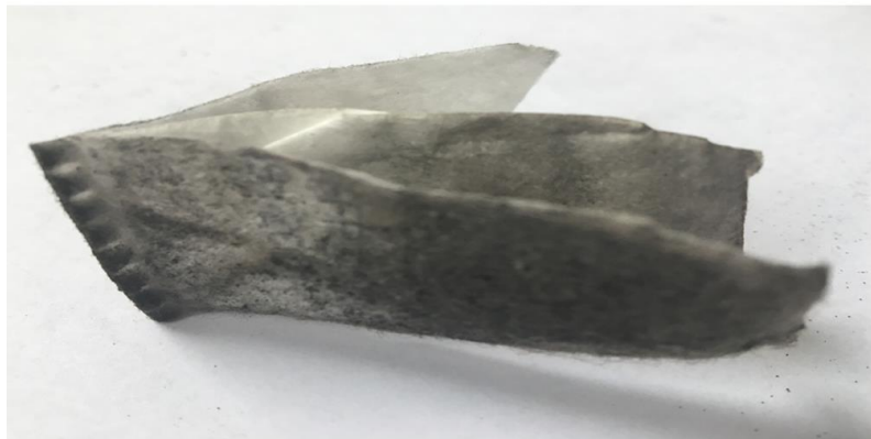
Fig. 1. Sample of filter from a half mask used during coal mining operations; the three layers have been partially separated, the outer layer in the foreground, then middle layer and finally inner layer
