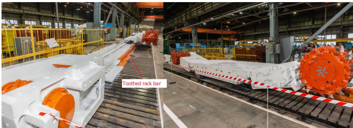
Fig. 9. The CLS550P shearer loader with electric haulage system with a toothed bar on the dedicated armoured face conveyor SPC271M from the coal face side [12]
