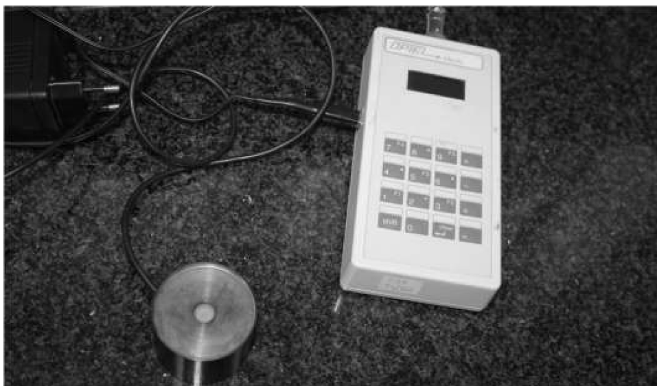
Fig. 2. Fito-photometer - device used to check power density
