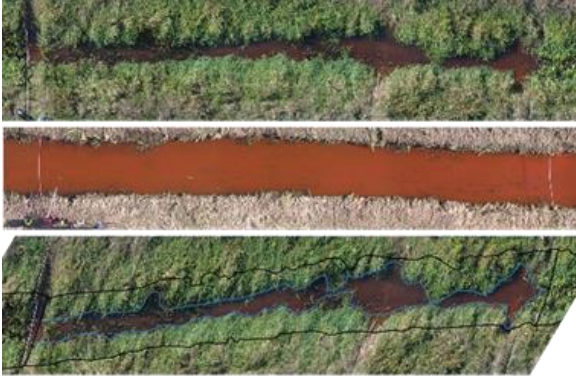
Fig. 2. Selected sub-reach in fully vegetated (top) and fully cut (middle) conditions during the passage of the tracer. The surface coverage of vegetation was determined by computing the ratio of the vegetation-covered surface area to the total wetted surface area available from the fully cut scenario (bottom) (after Västilä et al. 2021).
