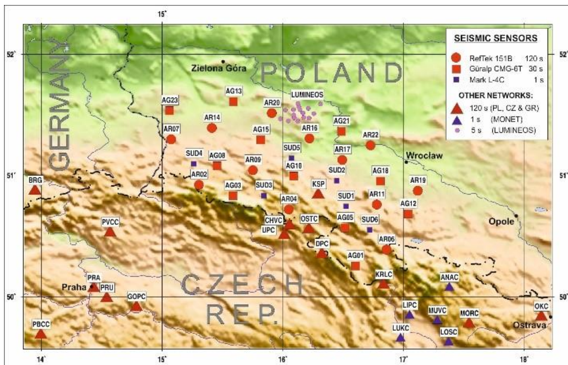
Fig. 1. Location of the seismic stations of the AniMaLS experiment in the Sudetes. Circles and squares – portable stations, triangles – permanent stations.
