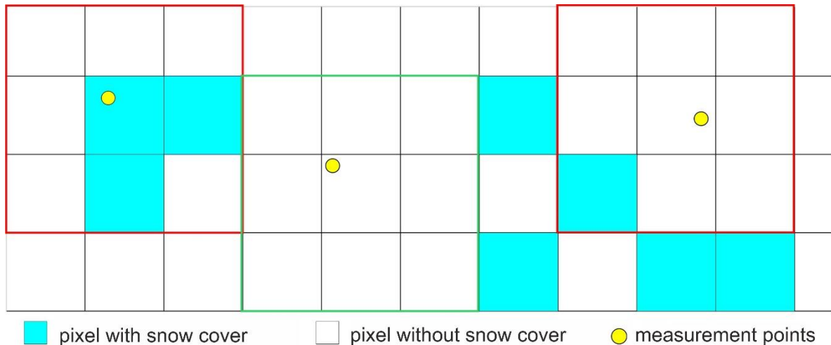
Fig. 38. The principle of determining the date of snow disappearance at the measurement site. In the above case, the middle point is considered snow-free.
