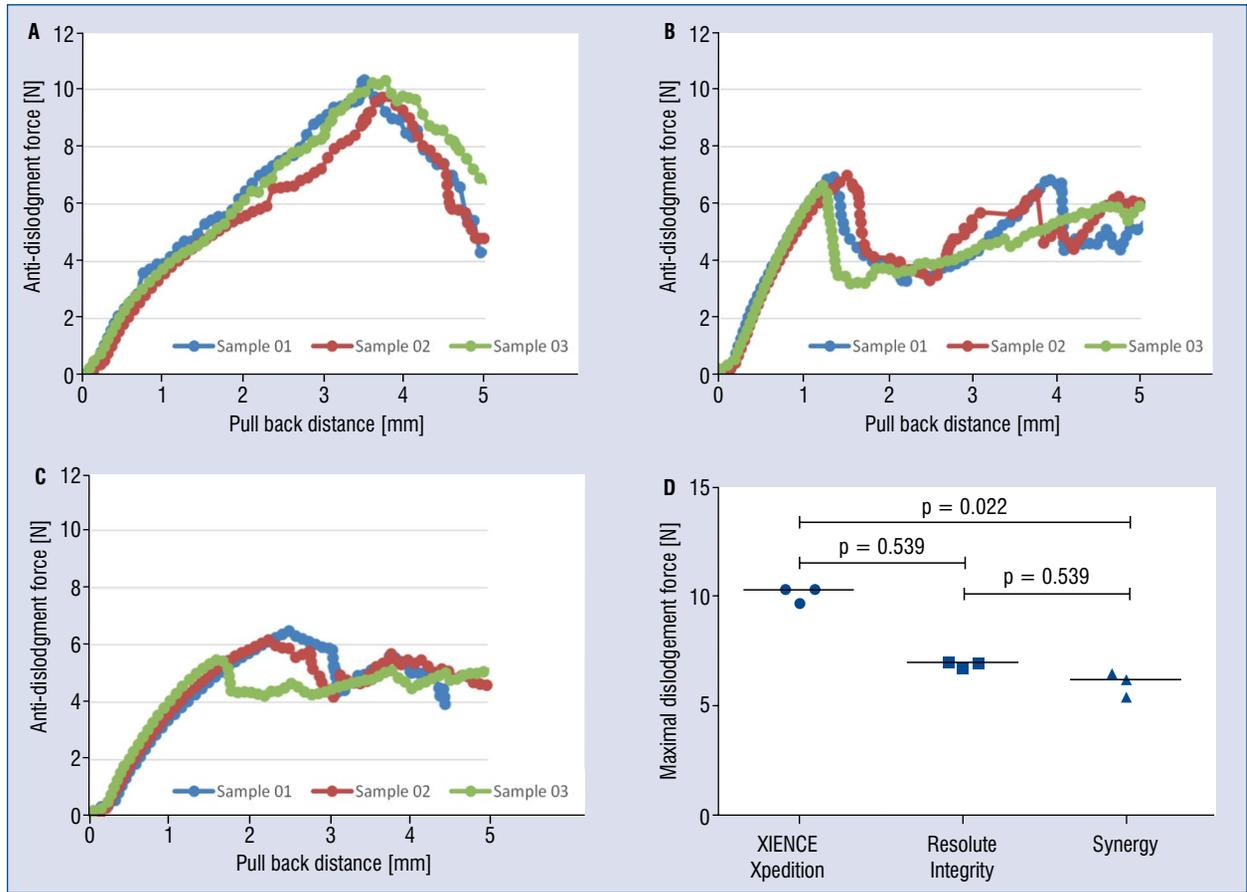
**Figure 1.** The values of force (N) during the pullback process for different drug eluting stents (with the speed of 50.8 mm/min). The force curves recorded in 5 mm pullback for XIENCE Xpedition (A), Resolute Integrity (B), and Synergy (C); D. Comparison of maximal dislodgement force among three drug eluting stents.
