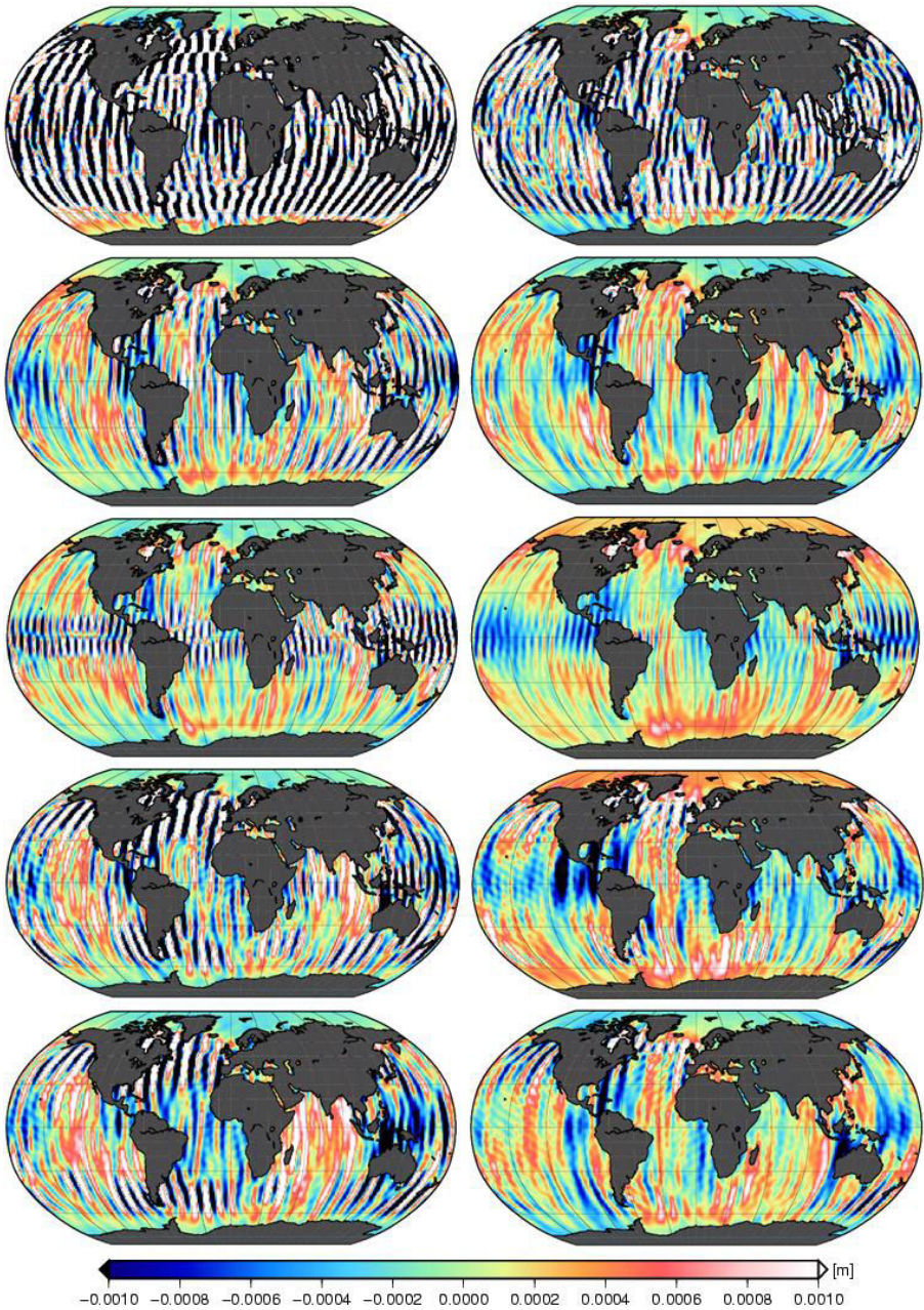
Fig. 7. Geoid height differences (in m) between the simulated static gravity field ITG-GRACE03s and the recovered solutions of the oceanic tidal aliasing case for the GRACE (left column) and pendulum (right column) mission scenarios according to the orbital heights from top to bottom: 407, 410, 412, 415, and 420 km.
