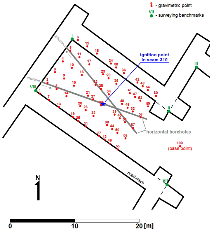
Fig. 3. Location of gravimetric measurements in the test site, Barbara experimental mine. In red – gravimetric points, in green – surveying benchmarks.
