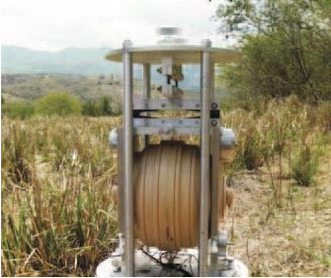
Fig. 1a. The suspended P-dIdD on a pillar. The outer spherical bias coils (D-coils) can be seen.
