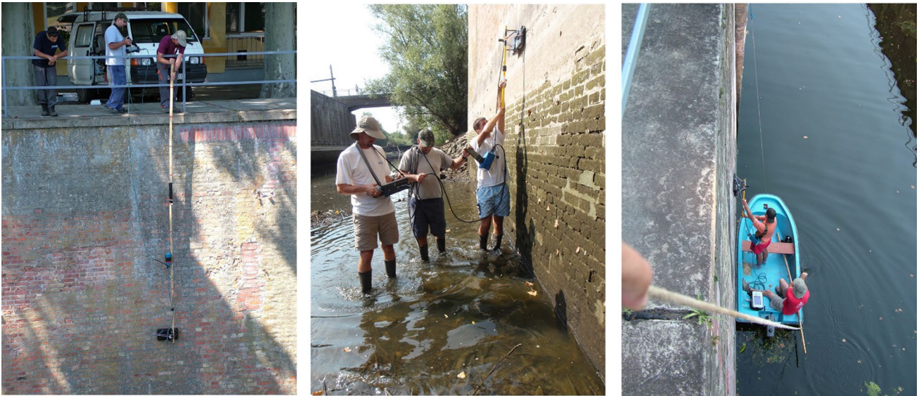
Fig. 9 GPR measurement using pole or boat
