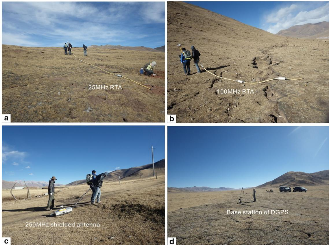
**Fig. 3** The composition of the GPR acquisition system and a differential GPS receiver mounted on the top of GPR antenna or the backpack. The GPR system is mainly composed of the center control
