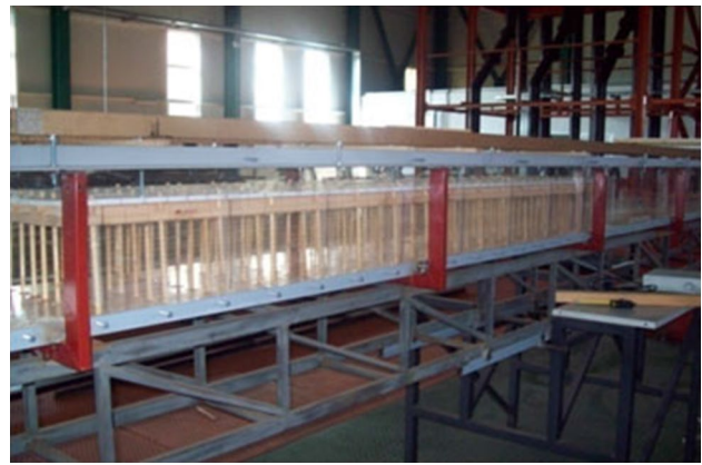
Fig. 2 Hydraulic flume with rod-simulated vegetation
