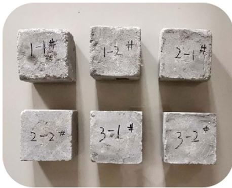
Fig. 2 Specimens with different mixing ratios
