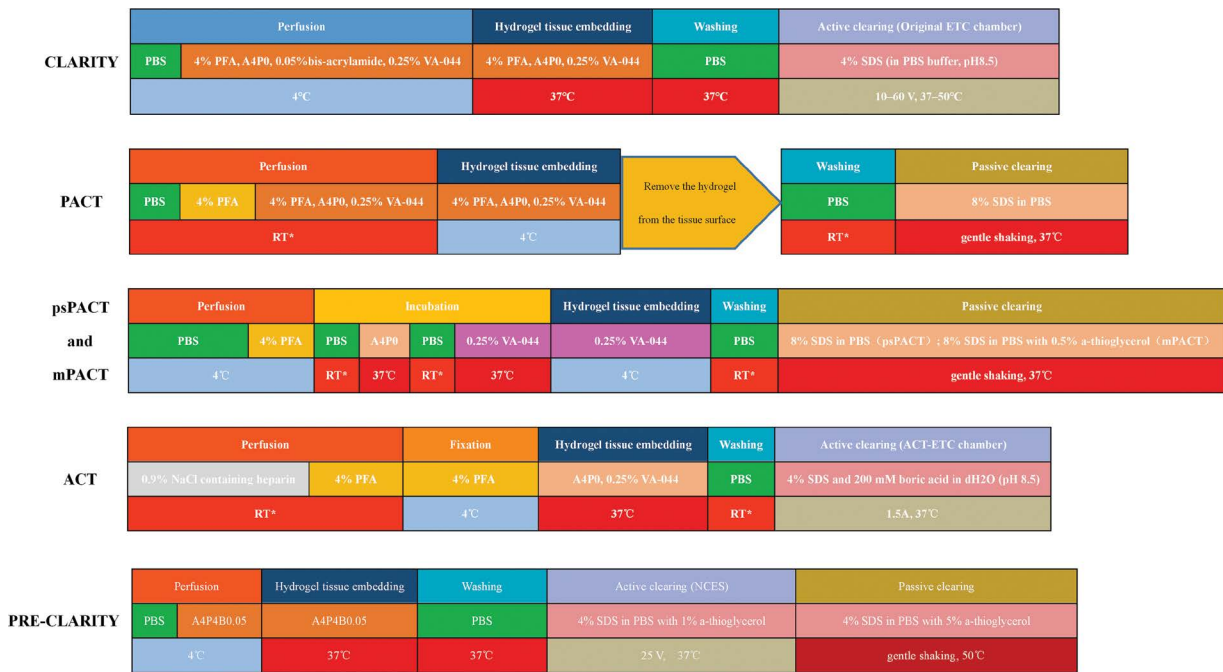
Figure 1. Schematic representation of CLARITY and its modifications. An outline of the individual steps involved in each of the CLARITY and its modifications is provided alongside the reagents required for each step. Each method has three rows of boxes. The first row presents the simplified steps of the protocol; the second row shows the required reagents; the third row displays the recommended working temperature; RT — room temperature; other abbreviations — see text.
