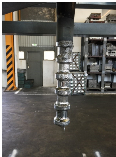
Fig. 2. Photograph of the stepped sonotrode used in the ultrasonic degassing tests
