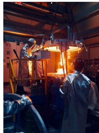
Fig. 3. Pilot plant induction furnace with lifted low pressure casting lid and casting pipe
