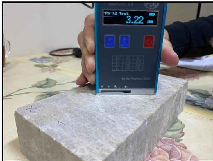
**Fig. 3.** Determination of surface roughness
