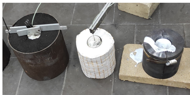
Fig. 1. Types of foundry mold used in the experiment: dry green sand mold, plaster mold, metal mold
