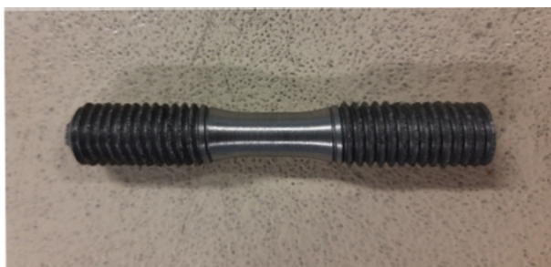
Fig. 3. Gray iron tensile strength sample made according to the customer's standard. Diameter of the sample D = 6 mm, length without fixings L = 15 mm
