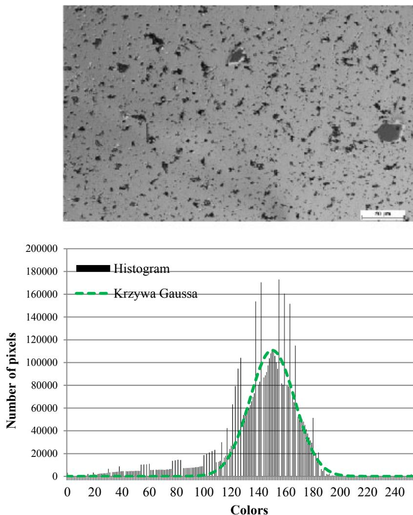
Fig. 2b clearly shows that in the case of this structure we can observe a much greater blurring of the histogram. This is due to the large number of point defects. The highest number of counts in this case is in the range of 120-180, which indicates the heterogeneity of the coating.
