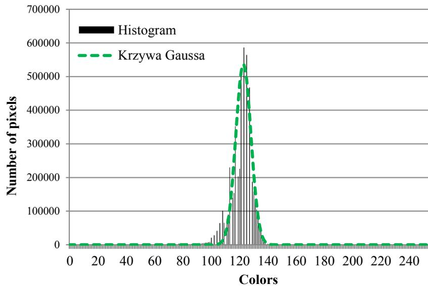
Figures 3a and 3b show that the structure P2 on silicon and glass is very similar. The layer on glass is homogeneous and has fewer point defects than the structure on silicon (Fig. 3a), but they are larger. The highest number of counts in the case of structure P2 deposited on glass is in the range of 110-135; the small range of greyscales indicates a good application of the coating on the substrate and confirms its homogeneity.
