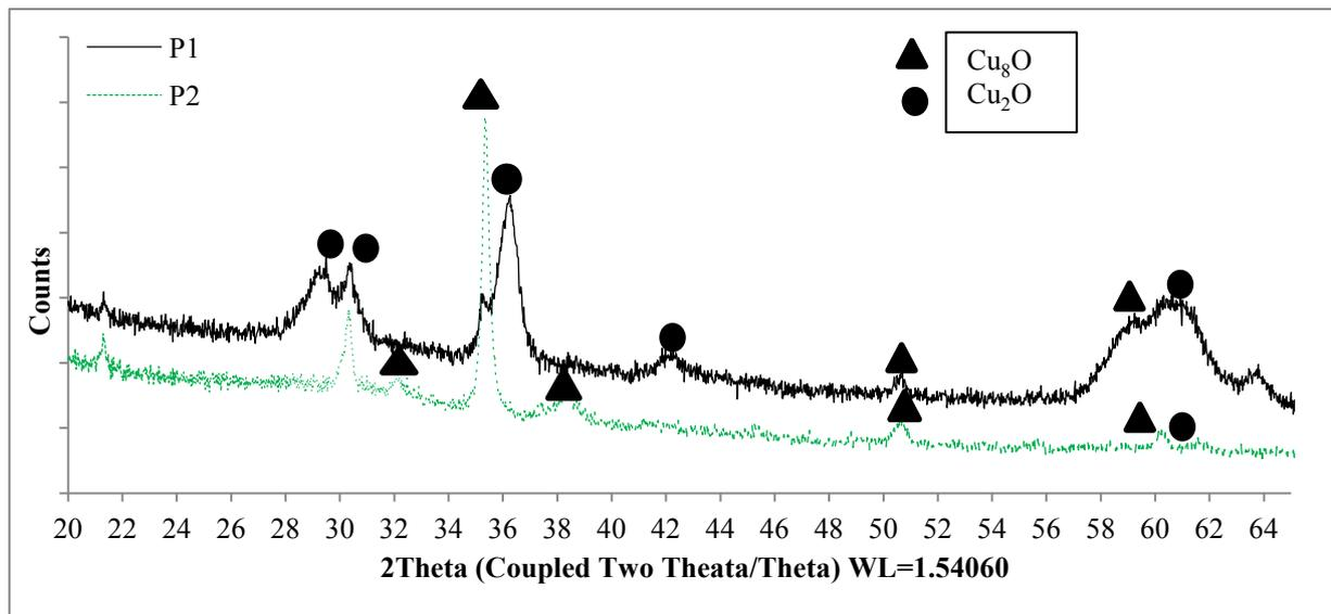
Figure 3. XRD spectra for  $\text{Cu}_2\text{O}$  samples deposited on silicon
