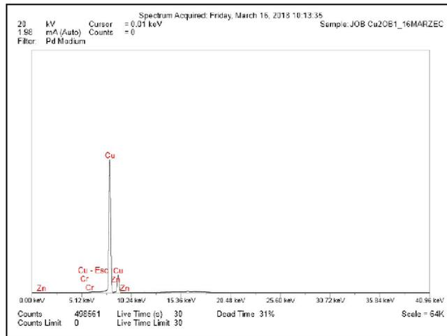
Figure 1b. Spectrum of elemental composition of the examined micro-area, layer on silicon, sample P1
