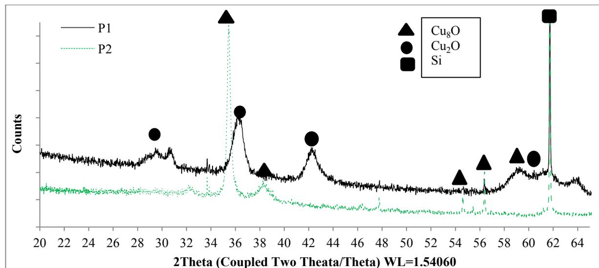
As the XRD diffraction graphs show, the structures differed significantly, indicating the influence of the preparation method. On the basis of the position of the diffraction line, it was found that they originated from phases  $\text{Cu}_2\text{O}$  and  $\text{Cu}_8\text{O}$ . Several researchers also reported  $\text{Cu}_8\text{O}$  in their study (Yonglong 2014; Guan, Hashimoto, Kuo 1984). Table 3 shows the phases detected, grain size, and the crystallinity and amorphicity of the samples.
