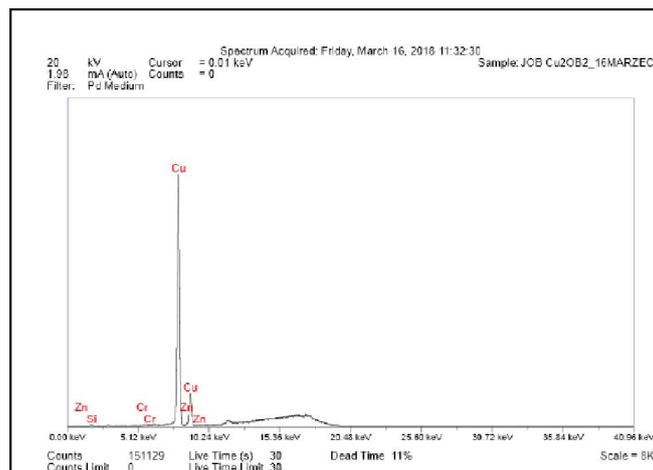
**Figure 1d. Spectrum of elemental composition of the micro-area under investigation, layer on silicon, sample P2**
