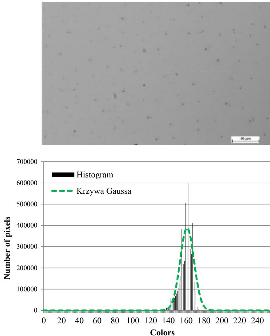
Fig. 2a. shows that the structure is homogeneous with a small number of point defects, which reflect the characteristic lines of the histogram. Its small blurring indicates the high homogeneity of the layer. The largest number of counts in this case is in the range 140-170.
