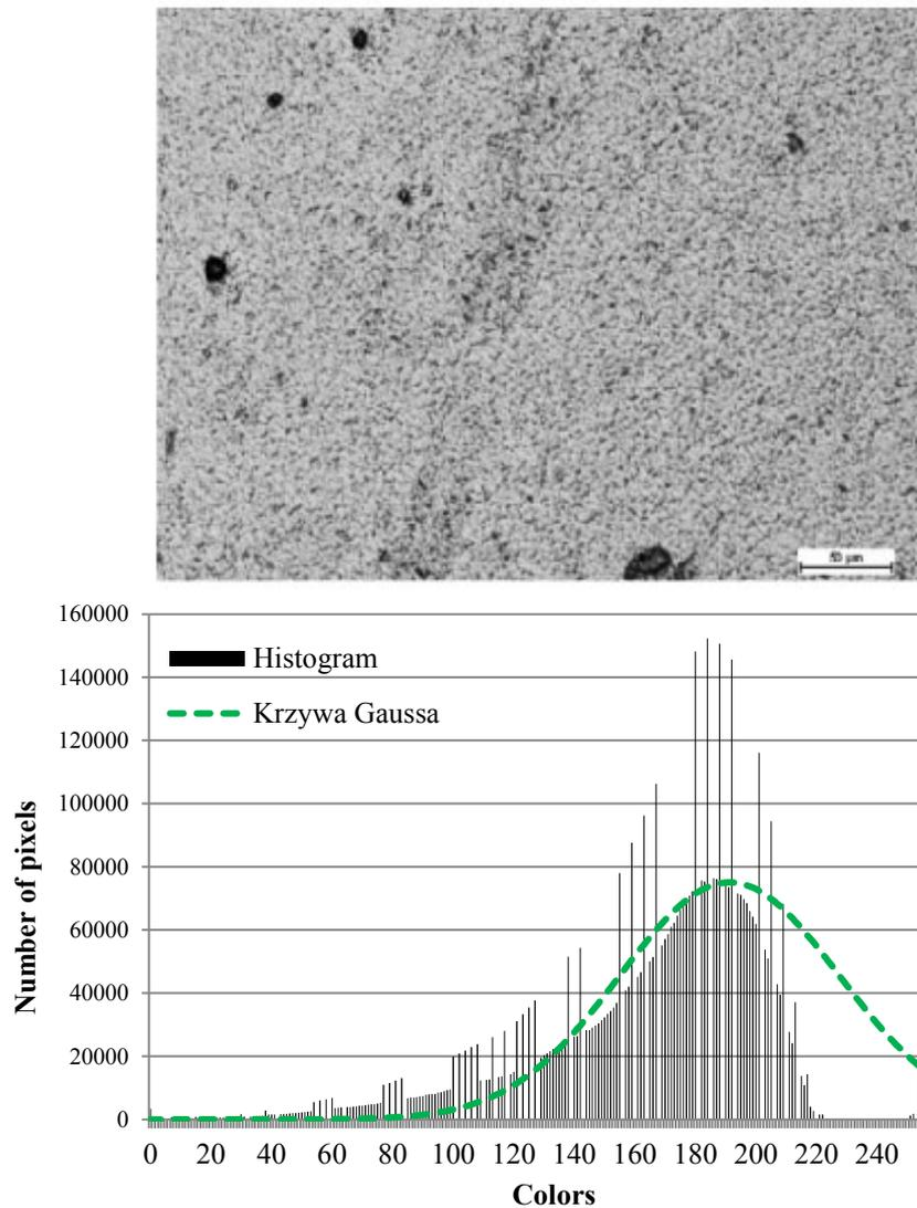
Analysing the image obtained during the examination of the coating with the optical microscope, it can be stated that, similar to the structure P3 deposited on silicon, the coating is fine-grained. From the histogram for layer P3 deposited on glass we can see that the layer is characterised by a large variety of surfaces. The greyscale counting range from 80 to 220 shows that there are many phases and surface defects. The largest number of counts in this case is in the range 150-210.
