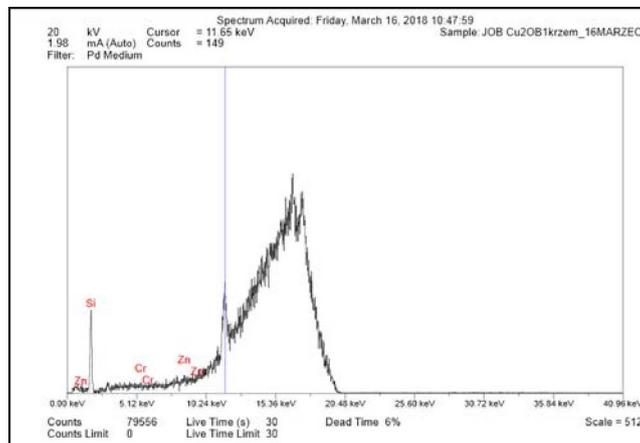
Figure 1c. Spectrum of elemental composition of the examined micro-area, layer on glass, sample P2
