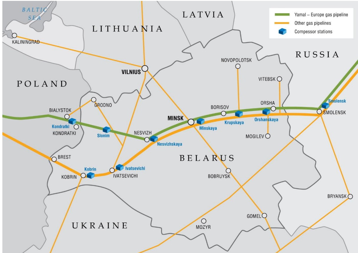
Figure 5. Gas trunklines in Republic of Belarus ( Gazprom, 2012 )
