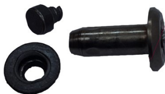
Fig. 5. Destruction of the MBF2110AB-05-15 rivet in a pull-off test
