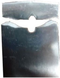
Fig. 9. Fatigue cracking of the central sheet of a double-overlap 32 mm wide sample
