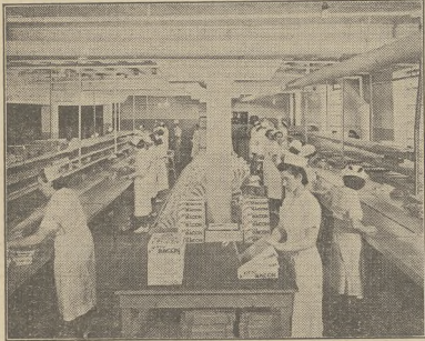
Modern bacon slicing operations. At the far end of the room are U. S. slicing machines, from which the bacon moves along to the weighers and packers in half-pound lots and then packed in cartons ready for shipment.
