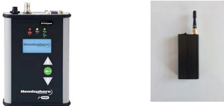
Figure 4. Devices applied to experiments: R110 receiver and Spy Electronic jammer. Source: authors' photo
