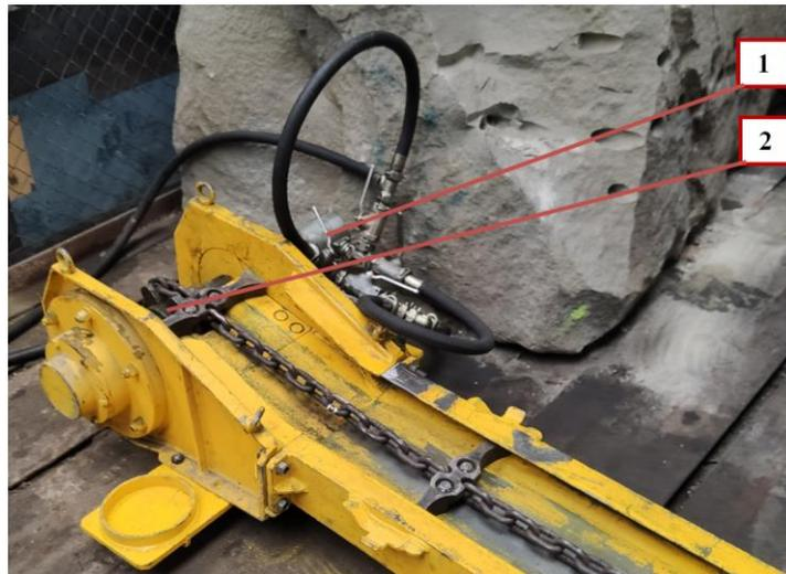
**Fig. 3.** Stand for testing dynamic forces – view from the drive wheel side, markings: 1- hydraulic motor, 2- drive wheel
