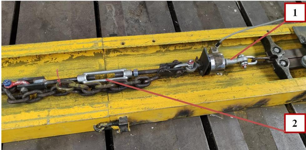
**Fig. 5.** Measurement sensors, markings: 1- force sensor, 2- turnbuckle
