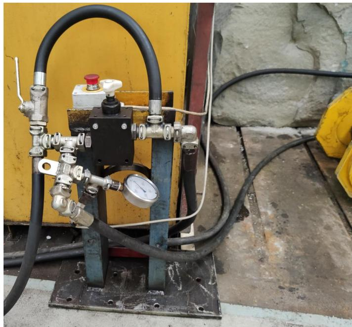
**Fig. 4.** Hydraulic control unit
