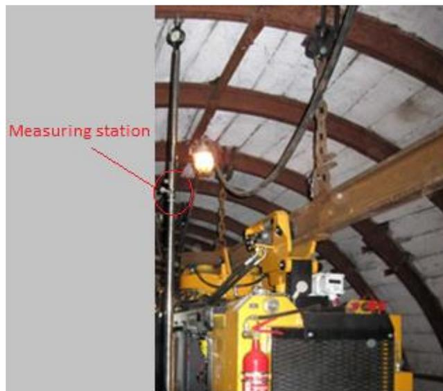
**Fig. 2.** Measuring station for recording the deformations of arch fastening during transportation of heavy loads
