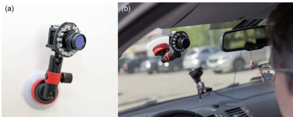
Fig. 2. Detector (a) ready to use and (b) located in the car cabin.
