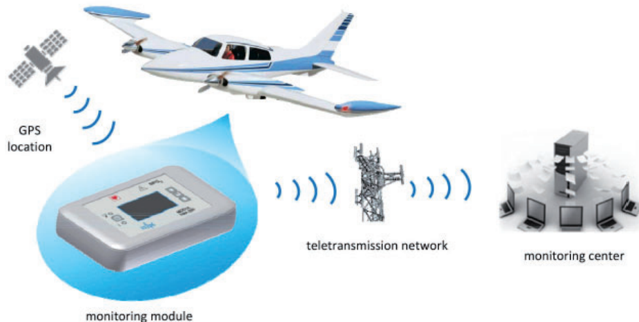
Fig. 8. SMP-3005 — System for monitoring psychophysiological parameters of persons during their professional activities.
