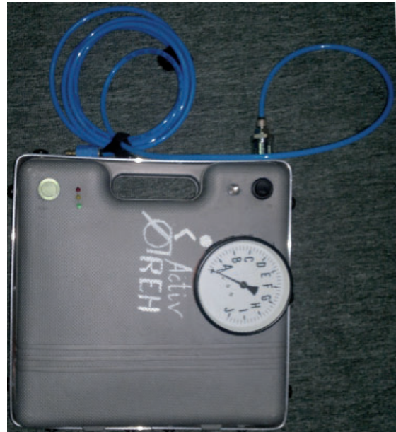
Fig. 8. The compressor for filling the R-WUK suit.
