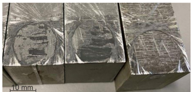
Fig. 8. Method of failure of samples whose upper elements were made of 2017A alloy with a diameter of 17.8 mm
