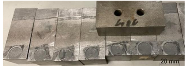
Fig. 12. Cohesive destruction of Raex 400 material samples with a diameter of 12.6 mm
