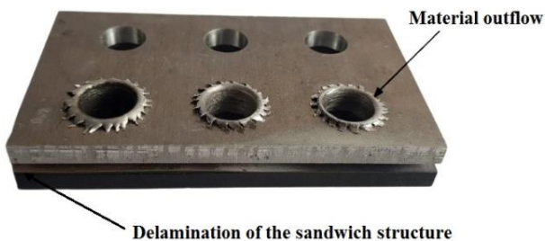
Fig. 4. Sample after drilling in the Al/CFRP strategy (pre-testing)
