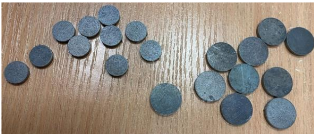
Fig. 2. Upper elements of block samples with diameters of 17.8 mm and 12.6 mm
