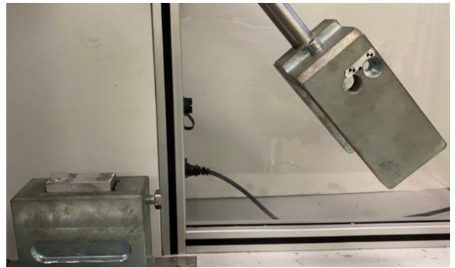
Fig. 6. Hammer prior to sample impact
