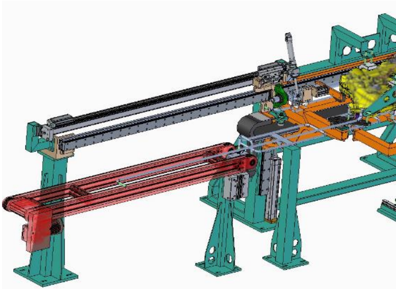
Fig. 8. Position of the feeder during tank loading
