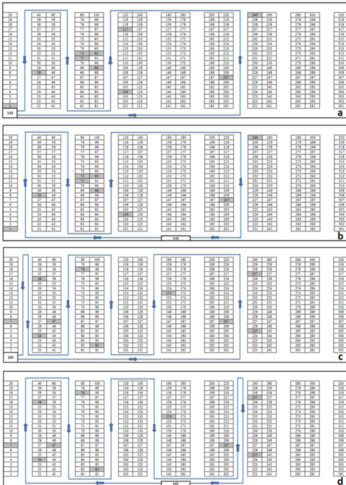
Fig. 1. Exemplary order picking paths a-b) for even and c-d) for odd number of (vertical) aisles to be traversed
