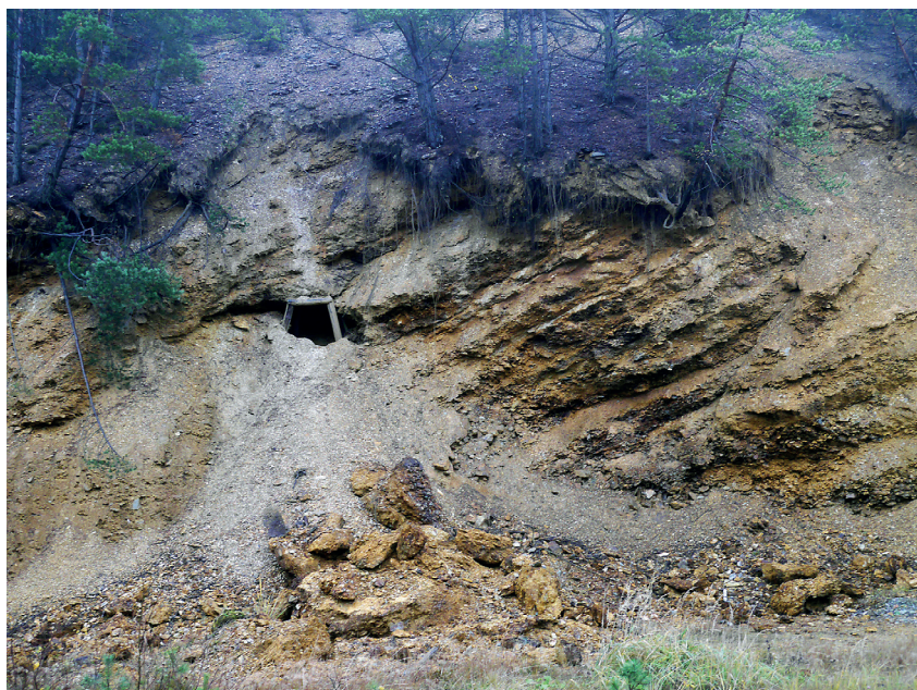
Fig. 32. Old heaps and galleries at Smolnik, used for the production of cementation water, photo P. Hronček
