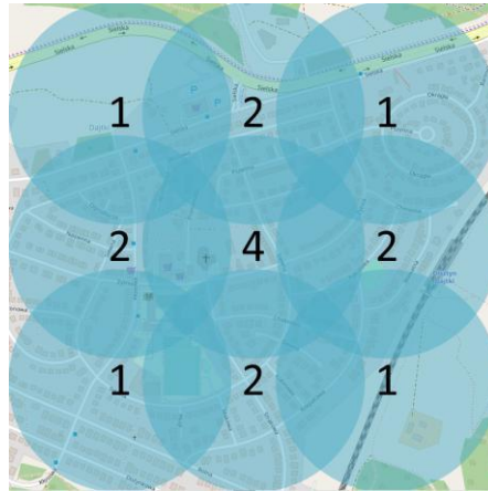
Fig. 5. The weights of individual neighboring units in Gauss filter discrete form for 3x3 kernel size and standard deviation equals 1 Source: Own elaboration on the OSM background
