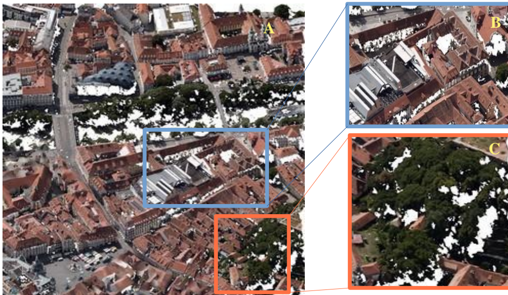
Fig. 11. Isometric view of 3D model from nadir images, (A – whole area, B – detail of building area, C – detail of urban vegetation) Source: own elaboration
