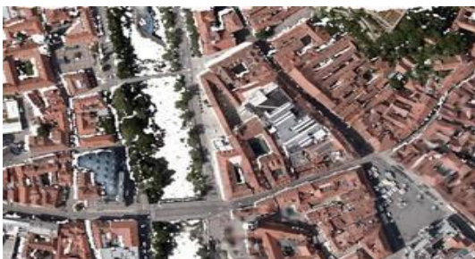
Fig. 7. 3D model from nadir images in orthogonal projection Source: own elaboration
