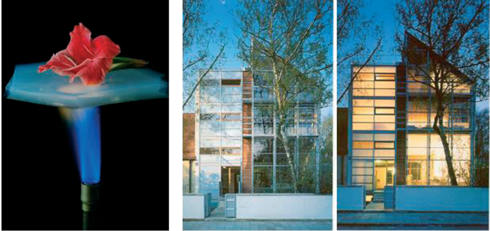
Fig. 6. Synergism in application: architect as a pioneer in using materials science developments. From the left to the right: a flower is on a piece of aerogel supported by the flame from a Bunsen burner; Public domain. Source: https://en.wikipedia.org/wiki/Aerogel#/media/File:Aerogelflower_filtered.jpg ; Translucent envelopes with high thermal resistance of the apartment building in Munich, Germany 1994, designed by Thomas Herzog, Architect; Source: Ashby M. Fernandez J. Unit 15. Architecture & Built Environment: materials for construction. Source: http://teachingresources.grantadesign.com/Architecture
