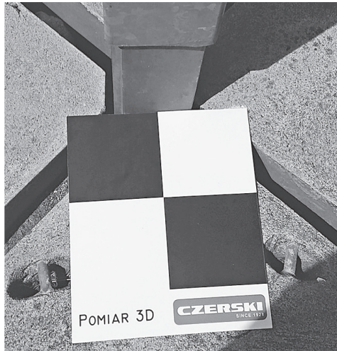
Fig. 5. View of example target plate used for matching point clouds into geodetic reference framework (photo by Krzysztof Karsznia)
