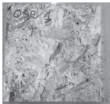
Fig. 6. Identification of the OSB 1 sample – 560 kg/m 3
