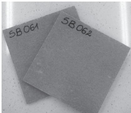
Fig. 3. Identification of the SB 061 and SB 062 samples. Insulating fibreboard – 240 \text{ kg/m}^3
