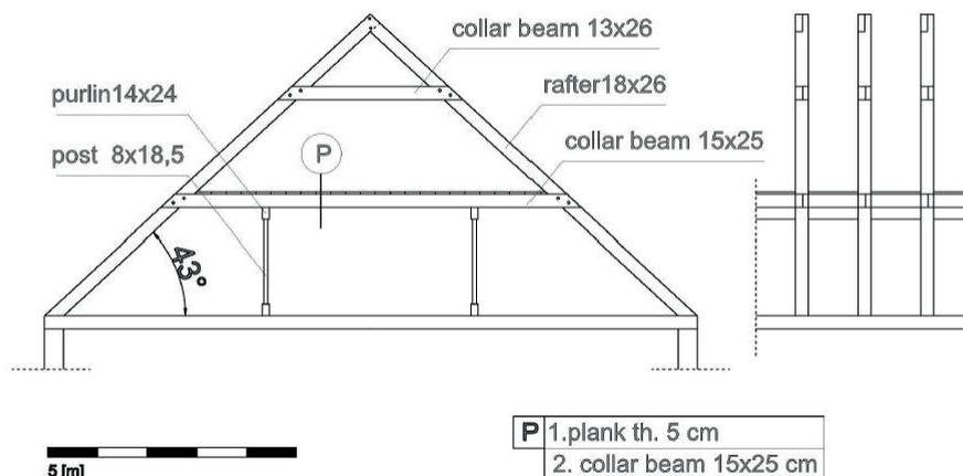
Fig. 12. The simplified scheme of the roof structure of the arcaded house in Marynowy. (author's study)
