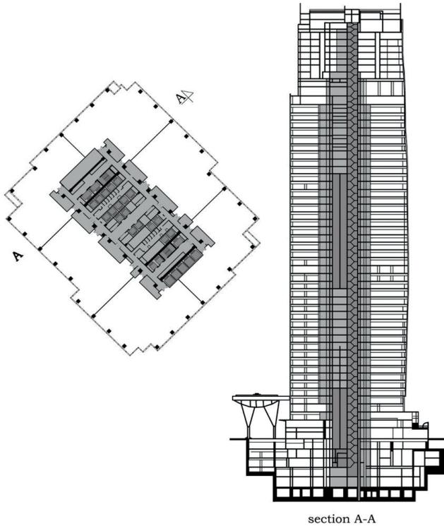
Fig. 12. Midtown Tower: floor plan and section, developed by authors [11]
