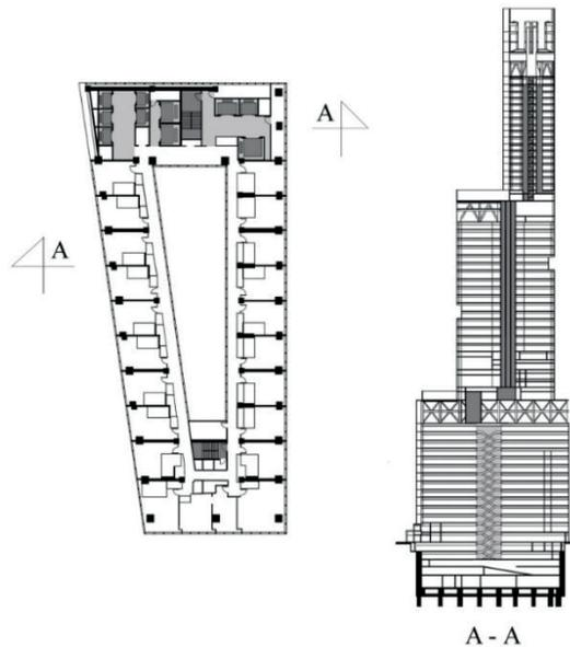
Fig. 8. Abeno Harukas: floor plan of the 53 and section, developed by authors [9]
