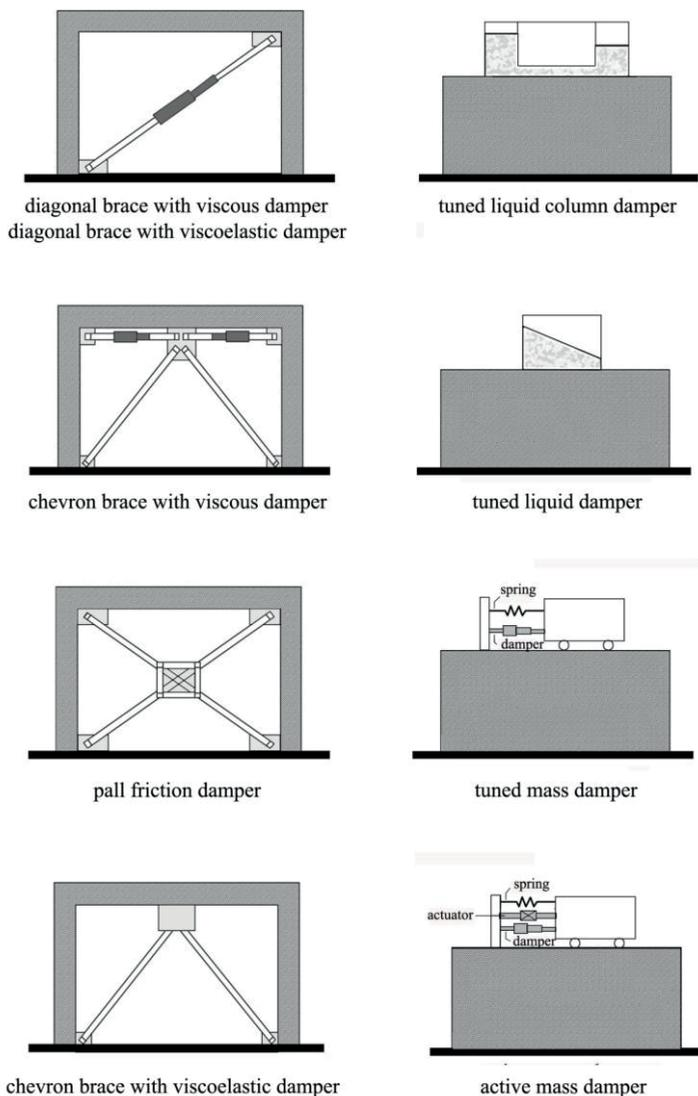
Fig. 6. Vibration damping systems (figure by authors)
