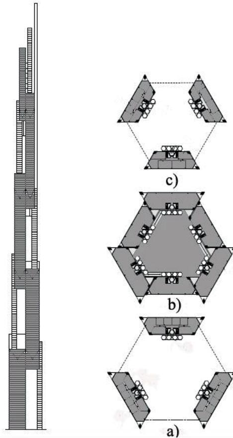
Fig. 4. Sky Mile Tower: floor plans (a) 1-35 floors; b ) 36-40 floors; c) 41-75 floors) and section, developed by authors [3]
