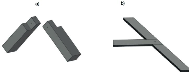
Fig. 6. Carpentry joints: a) lap joint , b) connection of collar beam with rafter with simple lap joint. (author's study)
