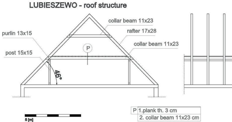
Fig. 21. The simplified scheme of the roof structure of the arcaded house in Lubieszewo (author's study)
