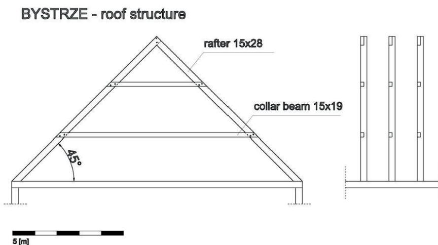
Fig. 9. The simplified scheme of the roof structure of the arcaded house in Bystrze. (author's study)
