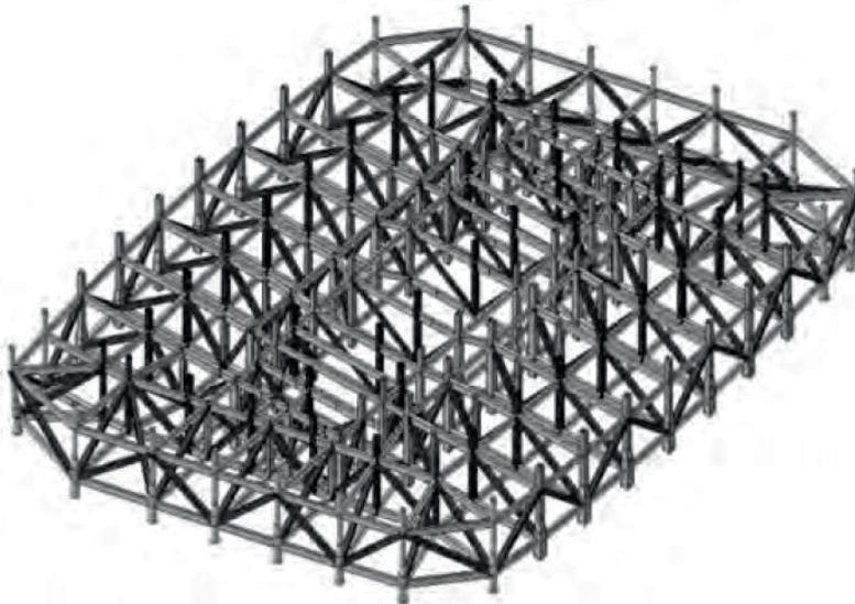
Fig. 16. Toranomom Hills: Structural spatial truss on the 36th floor [12]
