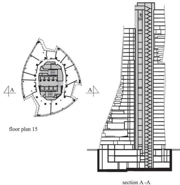
Fig. 24. Mode Gakuen Spiral Towers: floor plan and section, developed by authors [17]
