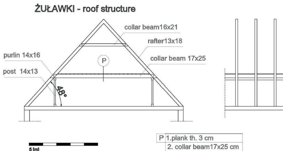
Fig. 22. The simplified scheme of the roof structure of the arcaded house in Żuławki. (author's study)
