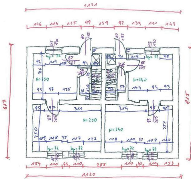
Fig. 4. An example of a manual sketch layout with dimensions
