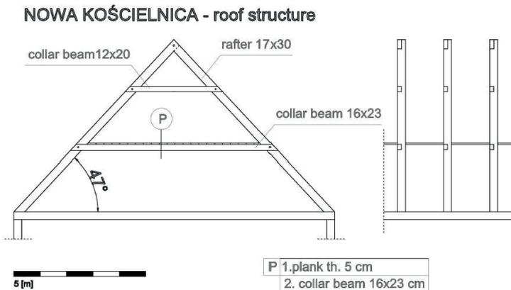
Fig. 15. The simplified scheme of the roof structure of the arcaded house in Nowa Kościelnica. (author's study)
