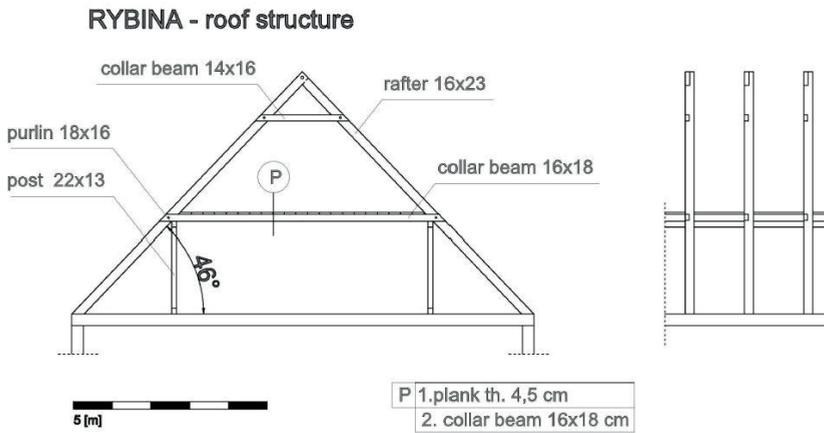
Fig. 18. The simplified scheme of the roof structure of the arcaded house in Rybina. (author's study)
