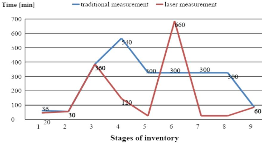
Fig. 6. Diagram of the comparison of the duration of measurements of individual stages - compilation by the author
