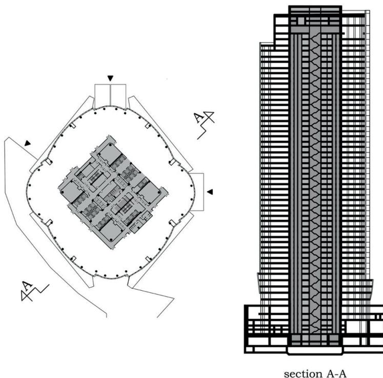
Fig. 18. Roppongi Hills Mori Tower: floor plan and section, developed by authors [13]
